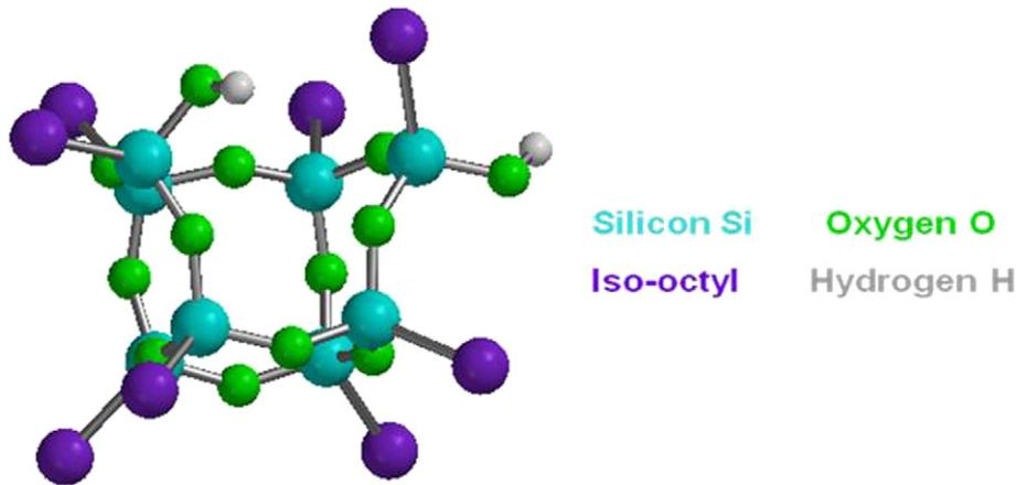
Fig. 5. Possible structure of the species  $T_8(OH)_2$ .
